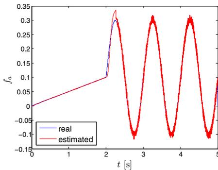
Fig. 3. Fault reconstruction with the LPV adaptive sliding mode observer.
