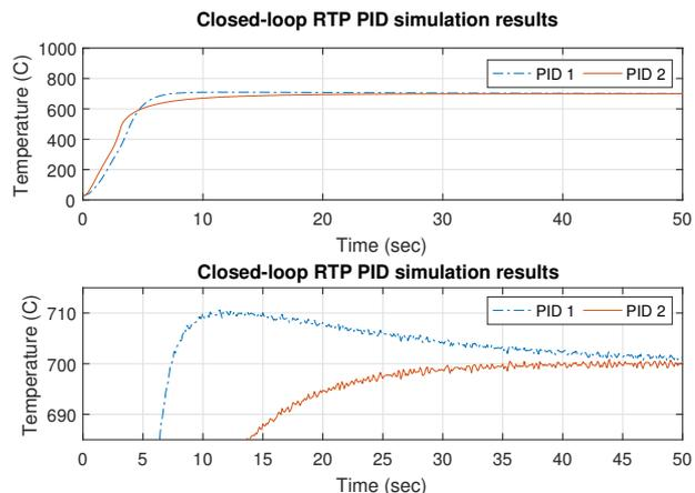
Fig. 7. Closed-loop response of the RTP system with two PID controllers: PID 1 allows overshoot while PID 2 does not (top: entire region; bottom: close-up).
