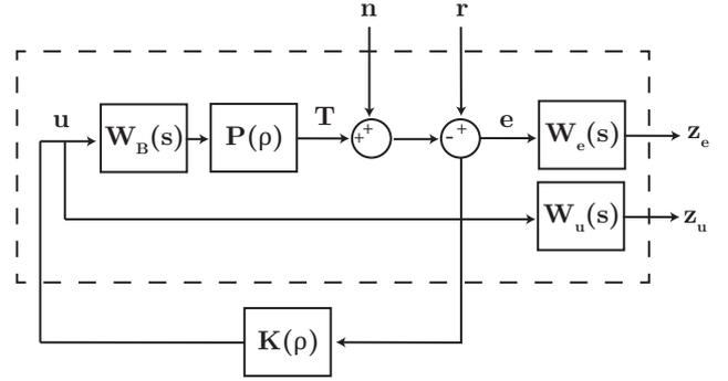
Fig. 4. Generalized configuration of the closed-loop system composed of the reduced LPV model, LPV controller, and loop-shaping filters.
