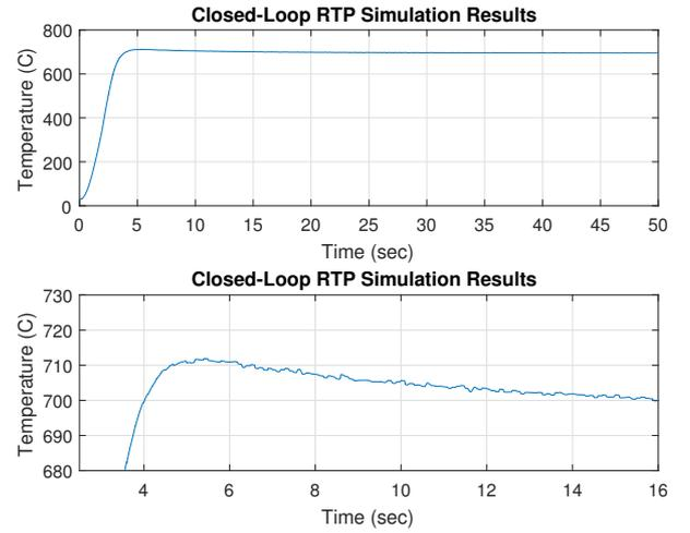
Fig. 5. Closed-loop simulation results for tracking a reference temperature (top: entire region; bottom: close-up on overshoot).
