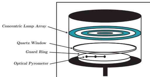
Fig. 1. Representative single wafer RTP setup.
