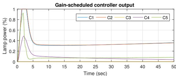
Fig. 6. Controller outputs of the gain-scheduled controller  $K(\rho)$  where  $C_1$  through  $C_5$  denote controller outputs corresponding to five zones.
