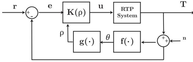
Fig. 2. Control of the RTP system using an LPV controller  $K(\rho)$  designed based on the reduced LPV model.
