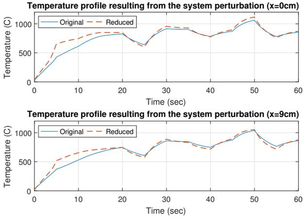
Fig. 3. Comparison between the low-order, low-scheduling variable model with the original nonlinear system. The top plot shows a node at the middle of the wafer, while the bottom plot shows a node at the edge of the wafer.
