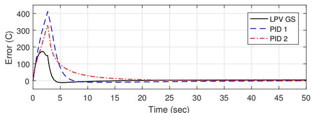
Fig. 8. Comparison between the error signals in the closed-loop response of the RTP systems using three controllers each tracking the same ramp input. The LPV GS controller clearly shows a better performance in terms of reaching the target much faster with less than half overshoot compared to the two PID controllers.
