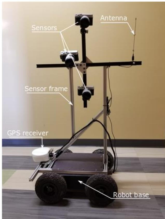
Fig. 1. Overall design of the robot. All other components are inside the robot base. The sensors are three color cameras.
