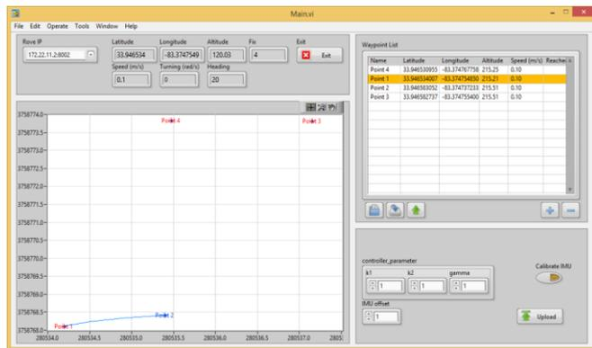
Fig. 4. Front panel of the PC program to monitor the robot.
