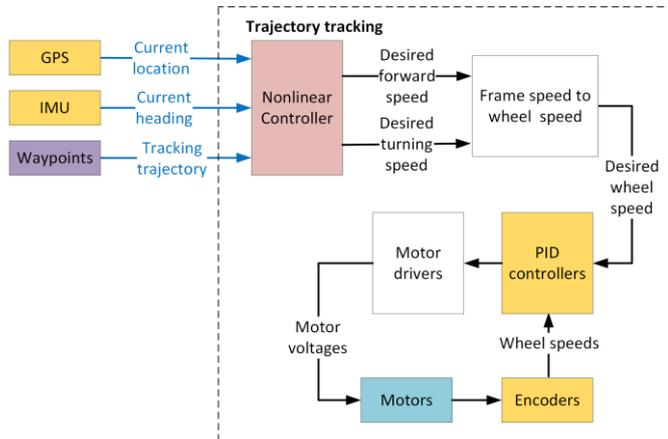
Fig. 3. Diagram of the autonomous navigation system
