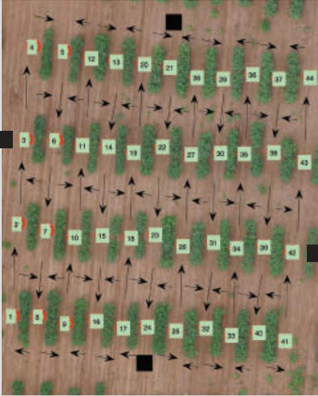
**FIGURE 2** The map of agricultural field: Image is captured by a UAS and the map is constructed using MATLAB. The black arrows indicate the allowed motion in each region and constrain the direction of movements of the robots. Numbers indicate the nodes of the corresponding graph.
