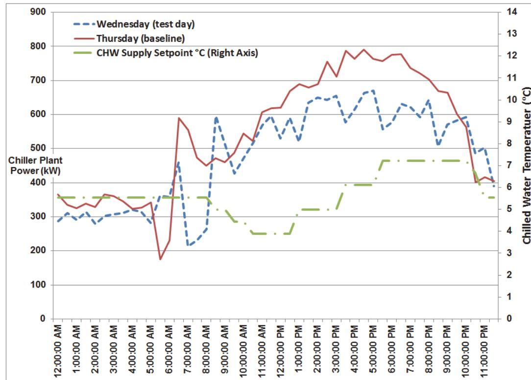
**Figure 4 – Results from Simulated Demand Response Testing, August 2015**
