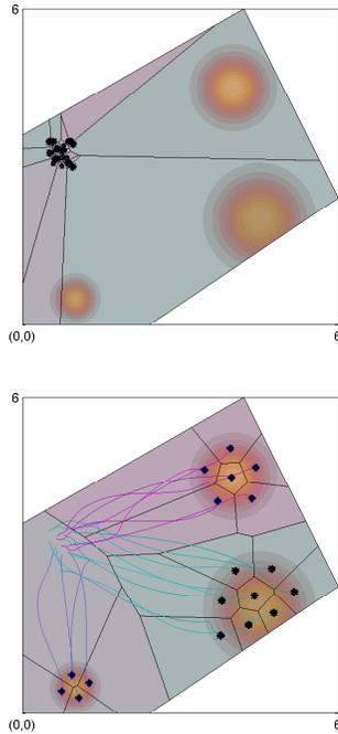
Fig. 3. Initial (top) and final configurations (bottom) for three groups of 8, 4, and 6 agents, each of which is deployed to cover a region of interest. The results show the flexibility of the proposed approach to cope with problems, where there is a need to assign various number of robots to different regions.
