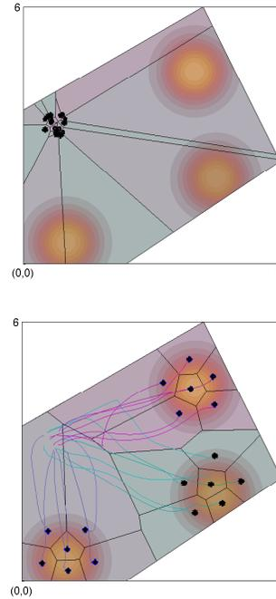
Fig. 1. Initial (top) and final configurations (bottom) for three groups of six agents, each of which pursues a different coverage task.
