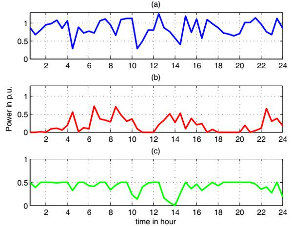
Fig. 6. (a) power generated by wind turbine and battery; (b) power generated by micro gas turbine; (c) battery state of charge
