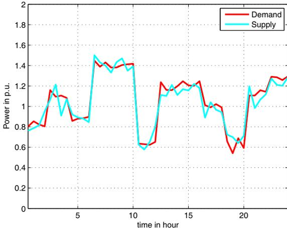
Fig. 5. Noisy load profile and optimized microgrid's total generated power (from wind turbine, battery and micro gas turbine)
