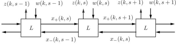
Fig. 3. Spatially-interconnected system in one-dimensional space.
