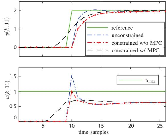
Fig. 4. Comparisons of the closed-loop response (upper) and control input (lower) at subsystem 11: unconstrained closed-loop system (blue), and constrained systems without (red) and with (black) distributed MPC.
