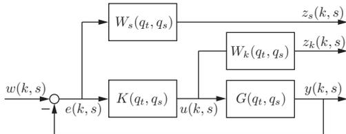
Fig. 2. Generalized plant for subsystem  $s$ .
