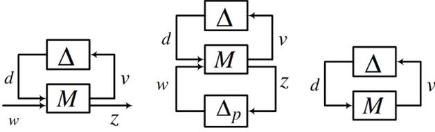
Fig. 4. Standard  $M-\Delta$  configuration: (a) for robust performance analysis, (b) with fictitious uncertainty  $\Delta_p$ , and (c) for robust stability analysis
