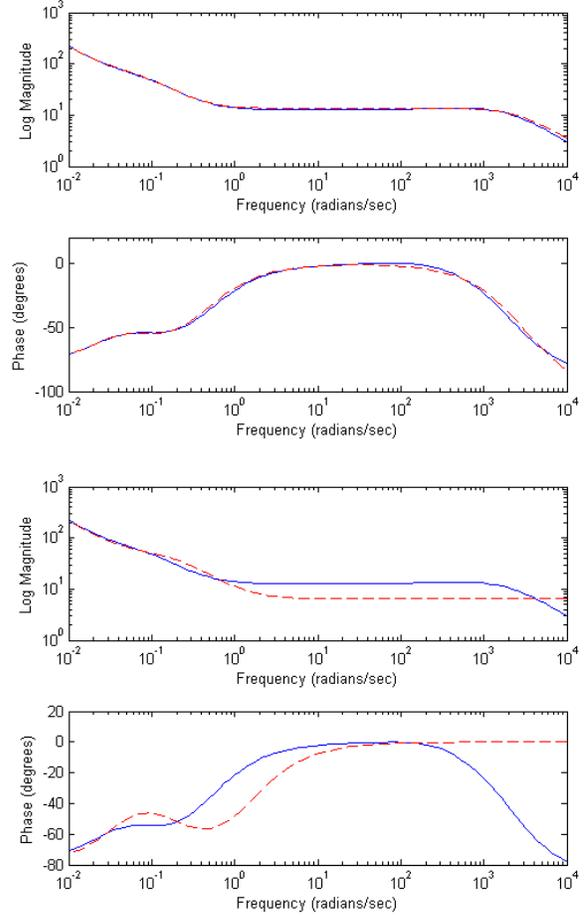
Fig. 5. Comparison of Bode plots of 14<sup>th</sup> order controller with that of (top) 3<sup>rd</sup> and (bottom) 2<sup>nd</sup> order controller.
