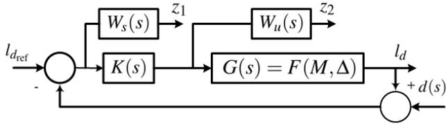
Fig. 2. Closed-loop system interconnection with controller  $K(s)$  and post-surgery patient described by the model transfer function  $G(s)$ ; variable  $d(s)$  represents measurement noise.
