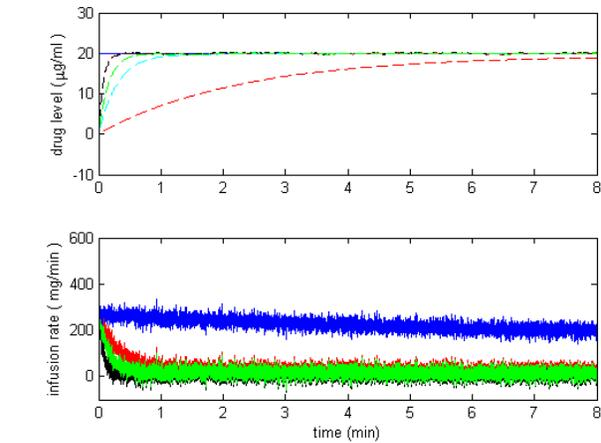
Fig. 6. Closed-loop simulation results for five randomly generated models of different patients showing: (top plot) controlled level of drug in patient blood plasma and (bottom) drug injection rate as the controller output.
