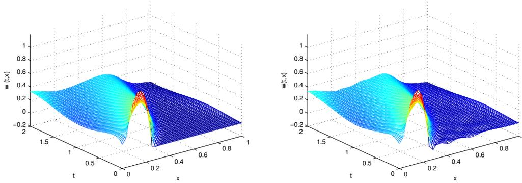
Fig. 2. Finite element solution for 32 spatial points (left), and POD solution with 7 basis functions (right) both with  $\nu = 0.01$ .
