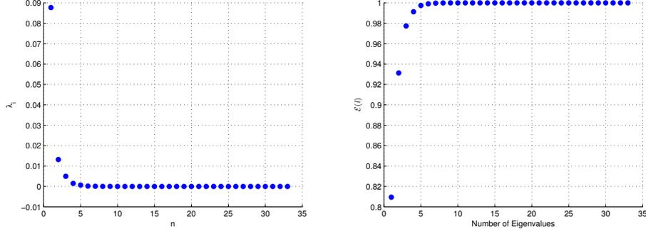
Fig. 1. The extracted eigenvalues corresponding to the POD eigenvectors (left); The energy captured by different chosen number of eigenvalues (right).
