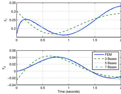
Fig. 3. The output of the FE model and the reduced-order model obtained using POD for different number of basis functions.
