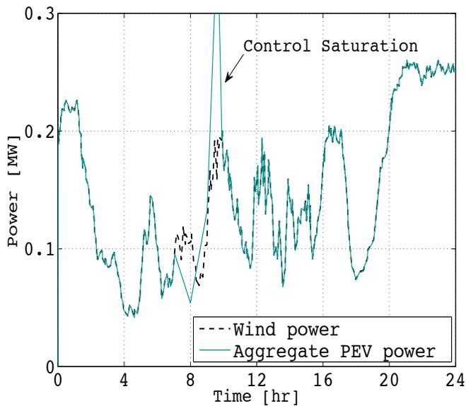
Fig. 6. Wind power tracking response for PEVs without anti-windup integrator
