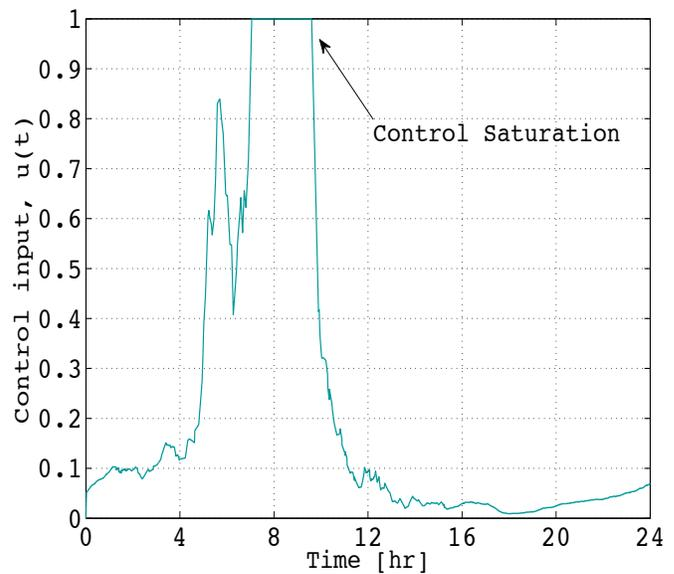
Fig. 7. Control input for PEVs without anti-windup integrator
