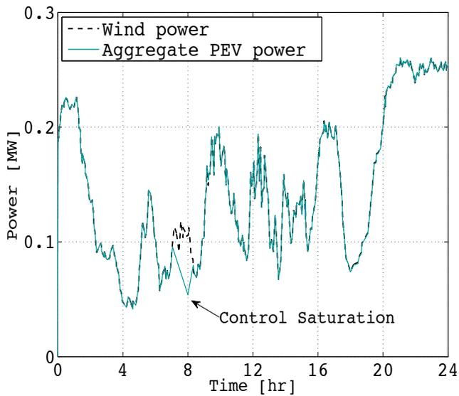
Fig. 2. Wind power tracking response for PEVs with anti-windup integrator
