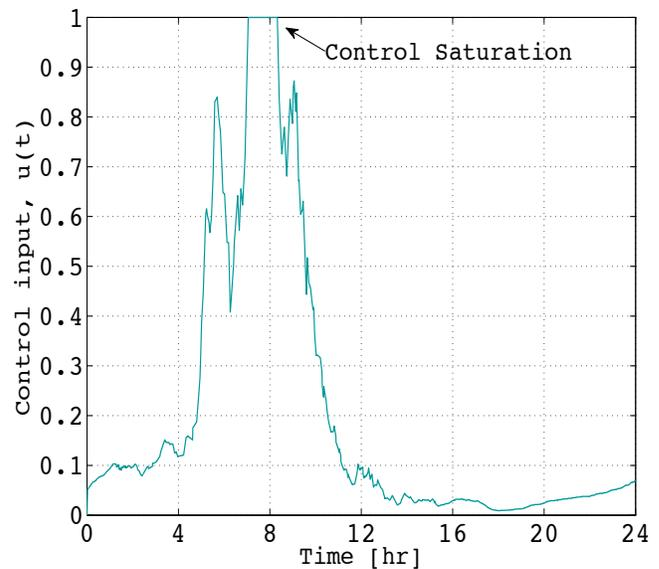
Fig. 4. Control input for PEVs with anti-windup integrator
