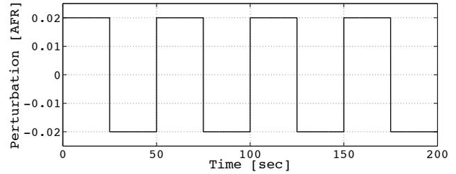
Fig. 3. Typical disturbance profile for the fuel injector and canister purge disturbance
