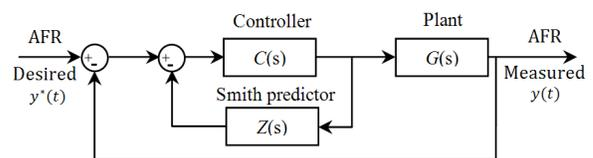
Fig. 5. A baseline PI controller with Smith predictor
