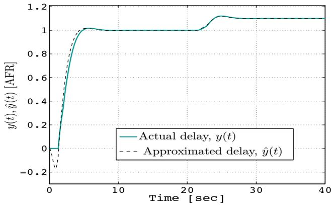
Fig. 2. Closed-loop system performance for the actual system,  $y(t)$ , and the approximated non-minimum phase system,  $\hat{y}(t)$
