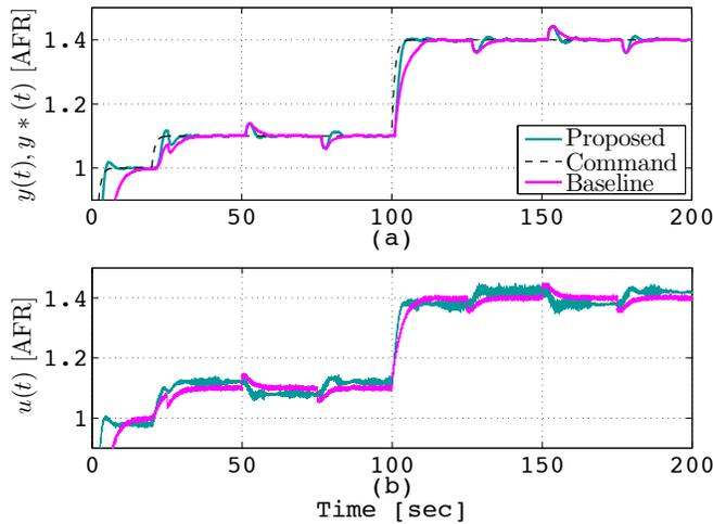
Fig. 6. (a) Output tracking with time-varying delay in the presence of the measurement noise and the fuel injector and canister purge disturbance; (b) The corresponding control input
