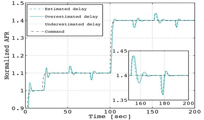
Fig. 4. Closed-loop performance in the presence of the fuel injector and canister purge disturbance and various delay estimation errors
