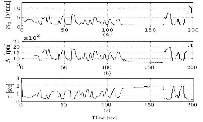
Fig. 1. (a) Air mass flow for the Federal Test Procedure (FTP), (b) Engine speed for FTP, (c) Estimated time-varying delay,  $\tau = \tau_c + \tau_g$
