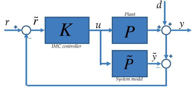
Fig. 1. Standard IMC design configuration for LTI systems
