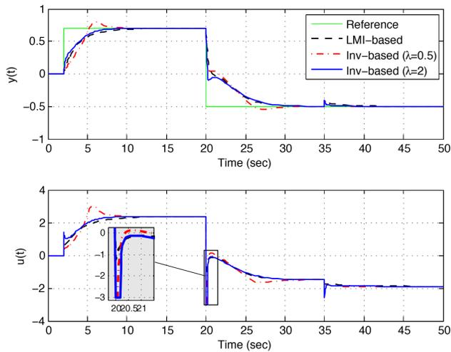
Fig. 2. Closed-loop system output response  $y$  and corresponding control input  $u$  for Example 1 using the two design approaches for IMC-LPV
