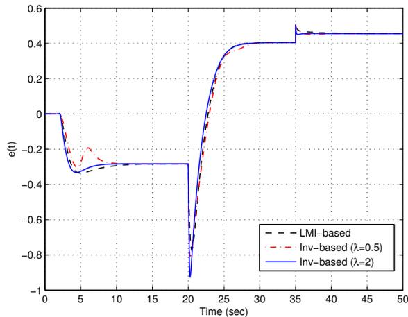
Fig. 3. Error signals corresponding to the three controllers for Example 1
