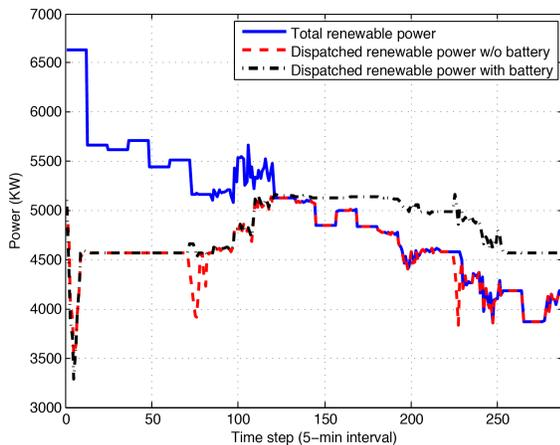
Fig. 6. Total available and dispatched amount of power from renewable sources with and without storage devices
