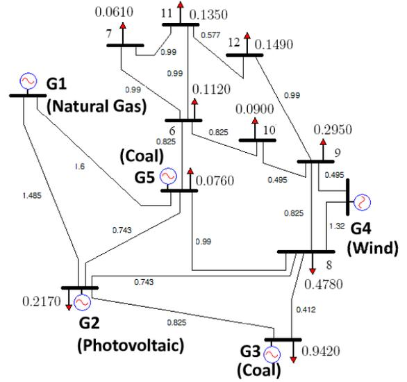
Fig. 1. Configuration of a 12-bus power network considering transmission line constraints and distributed loads (modified from [23])
