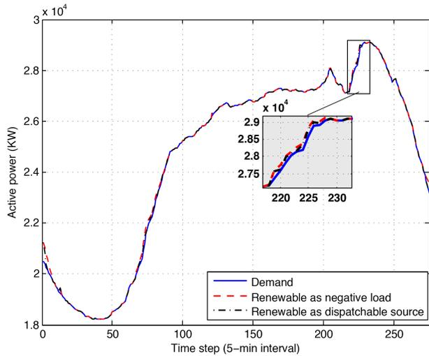
Fig. 3. Profiles of demand (solid line), total supply power considering renewable generation sources at buses 2 and 4 as negative loads (dashed line), and total supply power considering renewable generation sources to be dispatchable (dash-dotted line)
